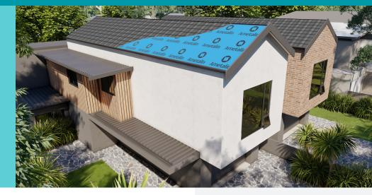
SilverSark® TRE - Tile Roof Extra radiant barrier is designed for use as a under tile roof sarking. It is suitable for use in all roofs. The reflective foil side provides extra R-value when installed facing an air cavity, and the multi-layer structure provides superior strength, flexibility and durability. Classified as a Water Barrier and Class 2 Vapour Barrier, SilverSark® TRE acts as a barrier to air, radiant heat, moisture ingress and dust penetration.
