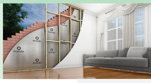
SilverWrap® Micro-perforated is an Extra Heavy Duty, Vapour Permeable wall wrap designed for use in brick veneer and drained cavity wall systems to reduce the risk of interstitial condensation in building systems. The reflective foil side provides extra R-value when installed facing an air cavity, and the multi-layer structure provides superior strength, flexibility and durability.
